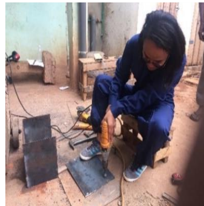
Figure 19: Drilling and leak testing the heat exchanger
