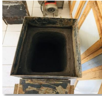
Figure 24: Kiln interior drying
