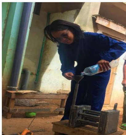
Figure 19: Drilling and leak testing the heat exchanger
