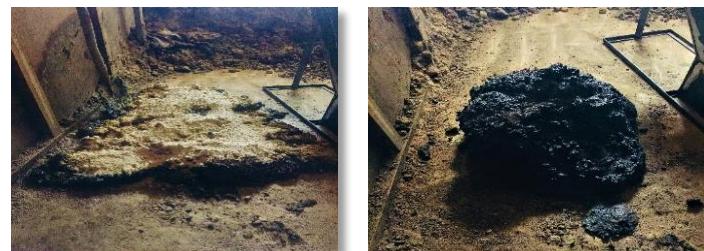
Figure 22: Clay + grog preparation and aging process
