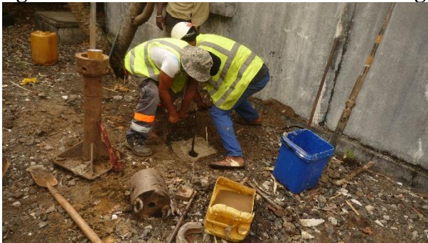
Figure 2. Soil reconnaissance tests using a Menard pressurometer
