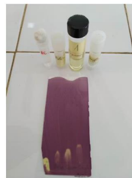
Graph III: Qualitative test by DPPH revelation on a TLC plate (a) in the TLC cuvette and (b) the reaction after DPPH revelation on a TLC plate with the samples to be analysed and an ascorbic acid control.
